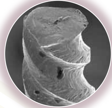
Micro-Cracks on Separated Instrument
