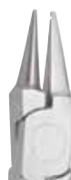
74-305 Light Wire Bird Beak with Groove For forming precise loops in light wires up to .020" (.51 mm). The groove in the tip allows for duplicating loops
