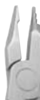
74-306 Tweed Loop Forming Loop forming pliers with .045", .60" and .075" (1.14 mm, 1.52 mm, 1.91 mm); For creating bull and helical loops in wires up to .022" x .028" (.56 mm x .71 mm)
